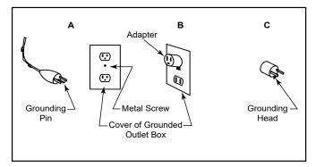
Figure 3.4 Cord Electrical Connection
