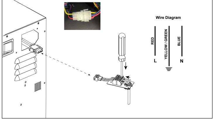
Figure 4.5 Wiring Hard Wire Terminal Block
