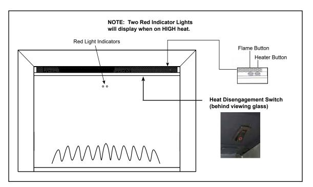
Figure 5.1 Manual Switch and Indicator Light
