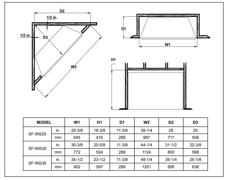
Figure 4.10 Framing Dimensions
